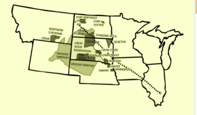
The 1,172-mile Dakota Access Pipeline (DAPL) is proposed to transport 470,000 barrels of crude oil per day (which is fracked and highly volatile) from the Bakken shale fields of North Dakota to Patoka, Illinois. Map courtesy of Camp of the Sacred Stones.
